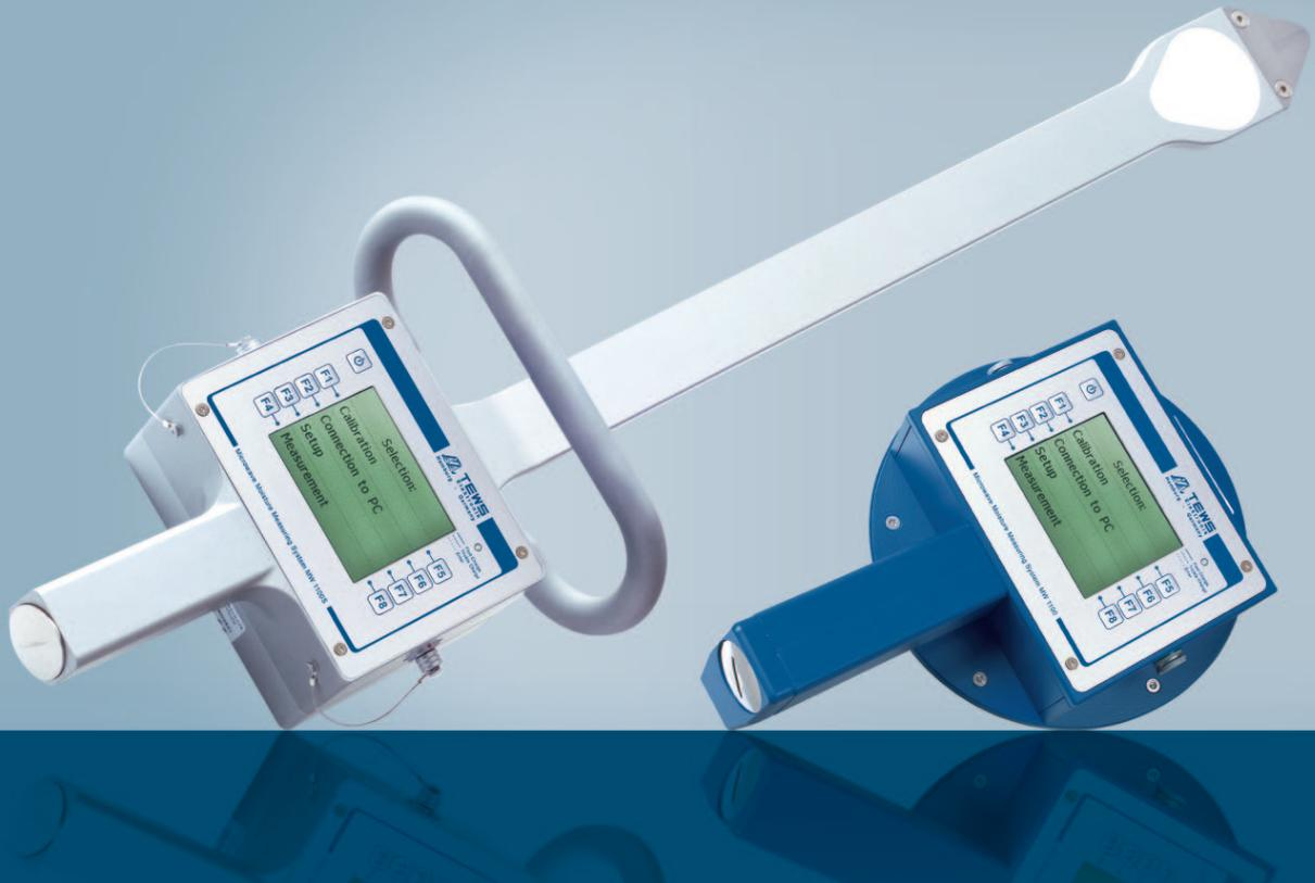
Portable moisture meters MW 1100 and MW 1100S are light-weight and handy models which allow operators to quickly and accurately monitor the moisture in a wide variety of products. They are intended in applications for manufacturers, goods receiving stations and quality control departments.
