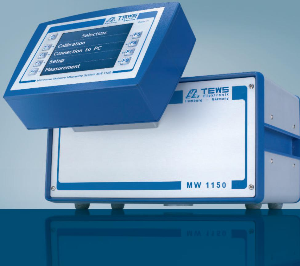
The MW 1150 is designed as a small compact laboratory instrument or atline instrument. It is based on the MW 11xx technology which allows readings within milliseconds to obtain sensor values quickly and reliably. The backlit 5.7" (14,5 cm) monitor displays the results - up to 250 readings can be stored in the system memory, atline applications use the standard 4-20mA interface to transfer values to a PLC. There are ports for a P 1150-type printer and various temperature sensors.
