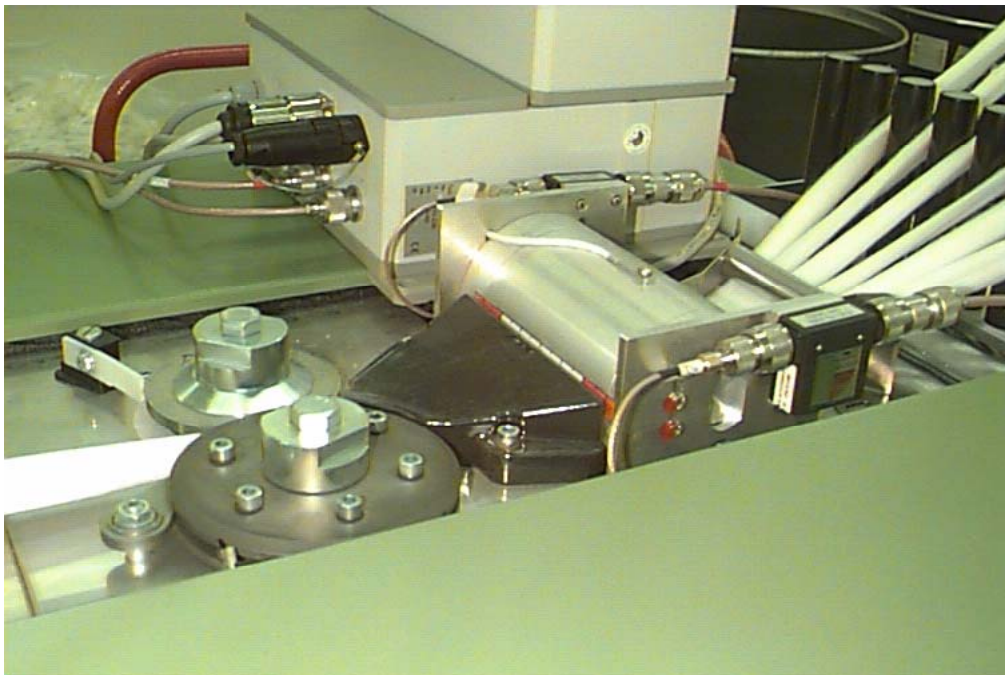
Fig. 5: Microwave measuring system and mechanical measuring system on a drawframe
